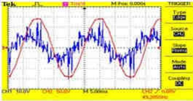
Fig. 7: Input & Output phase voltage at 30 Hz.
